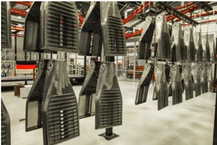
The alkaline two-component cleaner performs perfectly: the parts display a 100% hydrophilic surface. Photo: Henkel AG & Co. KGaA / Olaf Mündelein
