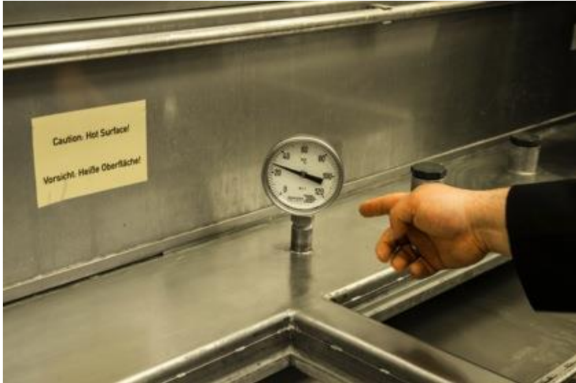
The low-temperature cleaning bath is not even at 30° Celsius. Photo: Henkel AG & Co. KGaA / Olaf Mündelein
